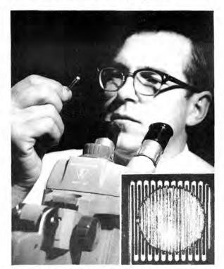
VERN BARR (8342) checks masking before manganin foil gage is plated to modify its physical definition. Inset shows gage grid after plating.
